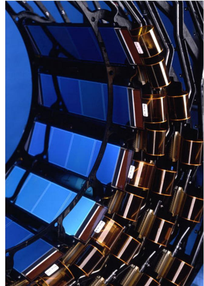
Strip or pixel detectors as inner trackers → position resolution
